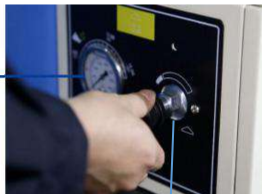
Figure 5.4: Turn clockwise to increase Pressure/Force the pressure, counterclockwise to decrease Adjustment Control decrease
