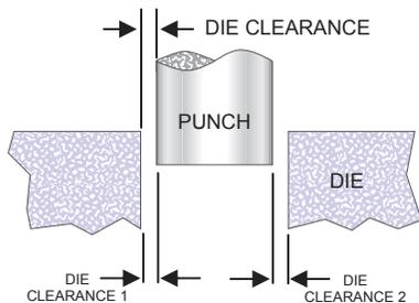
Total Die Clearance = Die Clearance on both sides of punch
