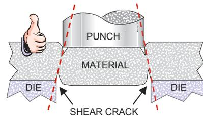
PROPER CLEARANCE - shear cracks join, balancing punching force, piece part quality, and tool life.
