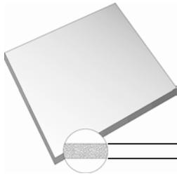
Material thickness is the width of the workpiece or sheet that the punch must penetrate in making a hole. Generally the thicker the material the more difficult it is to punch.
