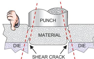
CLEARANCE TOO SMALL - secondary shear cracks are created, raising punching force, and shortening tool life.
